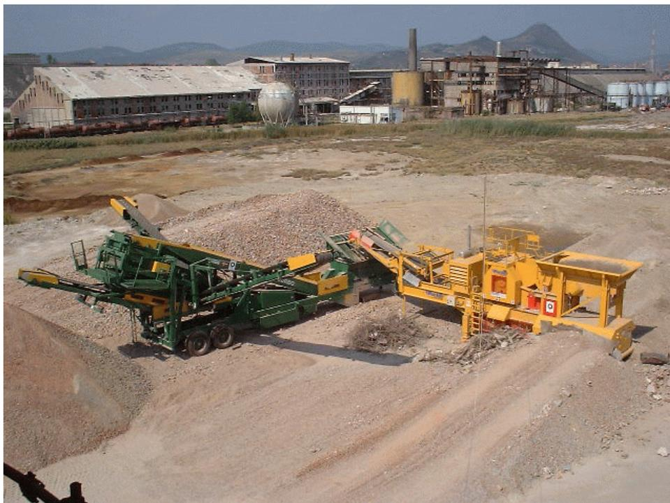
*Photo 19: A typical recycling depot with crusher and screener at an industrial site on the outskirts of a city (Mitrovica, Kosovo), on hard standing and with recycled materials stockpiled ready for collection. (Source: Golder Associates).*
