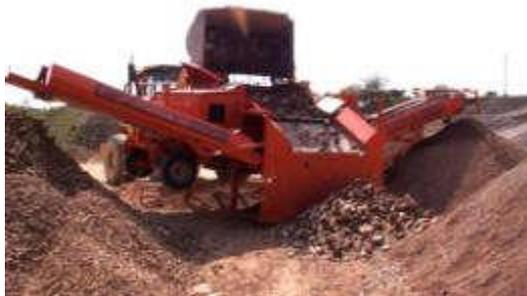
Photo 24: A primary screening feedstock for removal of soil fraction and possible contaminants (plastics, paper, non-recyclables) before crushing. (Source: Portafill)
