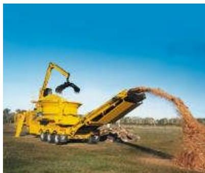
*Photo 28: A typical mobile shredding plant for green wastes such as timber and wood. (Source: Vermeer)*
