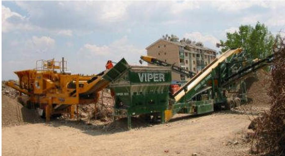
*Photo 27: Crushing of debris in Kosovo using a medium sized mobile crusher (yellow machine to the left in photo) and a screening unit for separation of the crushed material into 3 size fractions (green plant to the right in the photo). (Source: Golder Associates).*
