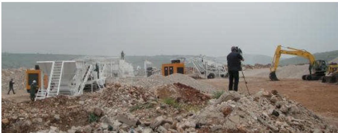
*Photo 1: The rubble recovery setup in Southern Lebanon as part of the UNDP Pilot Project. The photo shows (from the left) the manual sorting belt, the crusher and the screening unit with generators and one of the excavators employed. Source: MSB.*
