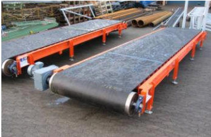
Photo 23: Typical conveyors with adjustable belt speed for use as a picking station.
